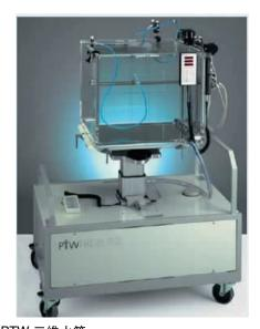
图 2 PTW 三维水箱 Figure 2. PTW Three-Dimensional Water Tank
